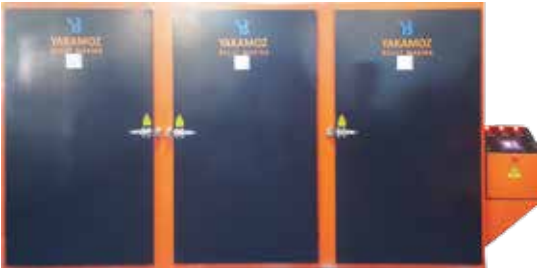
Brake pads/lining drying oven
