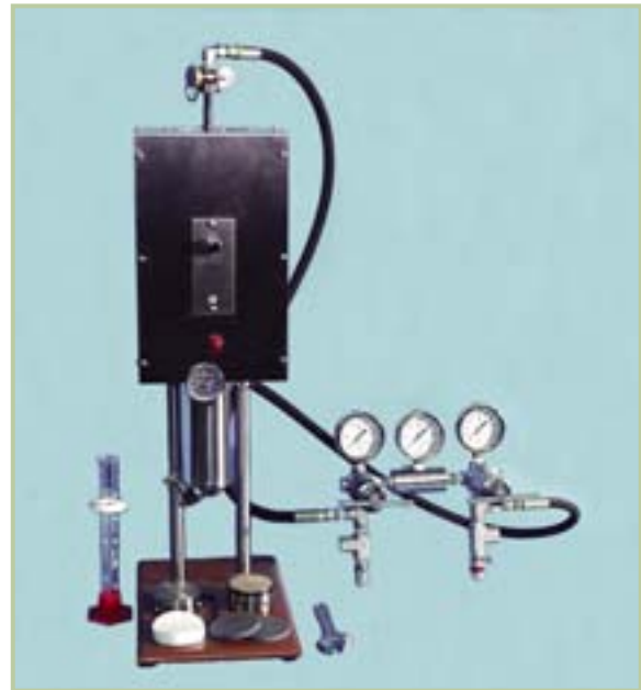
171 Series HTHP Filter Press with Nitrogen Manifold, 500 mL Ceramic Filter Disks and Extra Thick Cell Caps Optional
