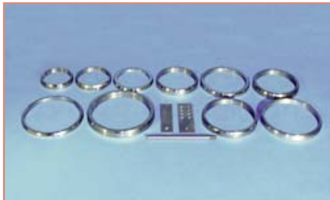
Corrosion Rings and Coupons
