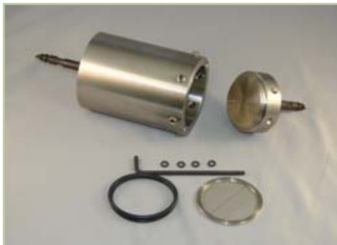
#170-45-1 Cell Assembly for Cement Testing
