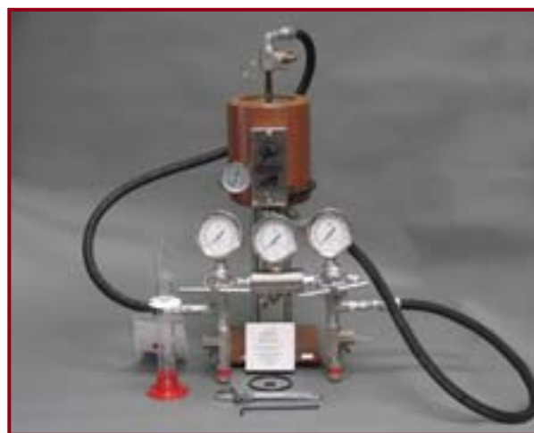
HTHP Filter Press with N 2 Pressure Manifold, 175 mL
