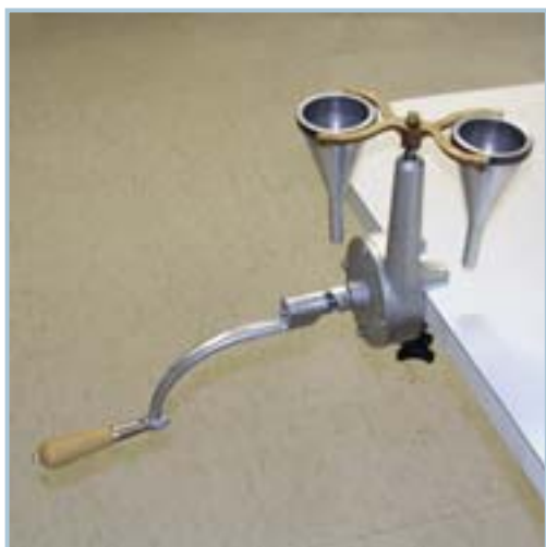
#153-25-1 Hand-Crank Centrifuge, 100 mL Capacity
